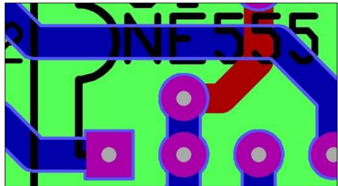
Figure 7 - Detailed view of engraving and cleaning tracks
