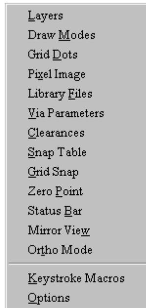
The Setup commands tell CIRCAD'98 how to draw a given file on the screen. You'll use Setup to name board layers, assign them colors, turn layers on and off, and so on.
